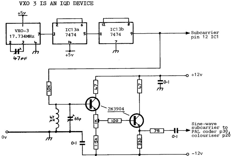
Fig.4 COLOUR SUBCARRIER OSCILLATOR (PAL)
