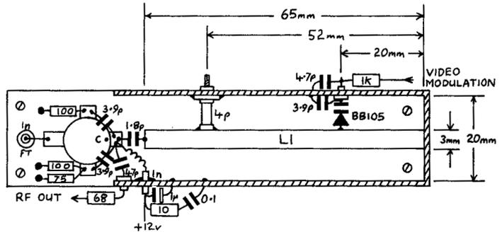
Trough made from copperclad PC board (good quality) or sheet copper or brass. Trough height is 20mm. Trough should be securely mounted and have good connections to ground. BB105 diode is tipped white and may be taken from ELC1043 types of domestic TV tuners.
