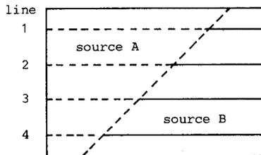
If this principle is extended it can be seen that a triangle field waveform will produce a wipe; and a triangle at line rate also will produce a diamond wipe.
