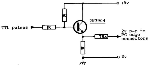
Fig.3 OUTPUT BUFFER - 1 FOR EACH PULSE OUTPUT
