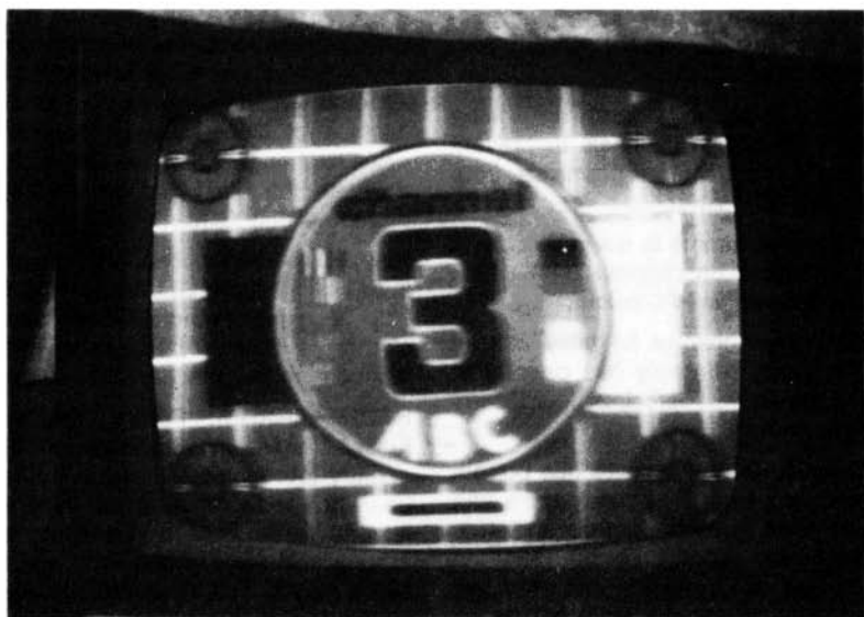
A Golden Oldie! An early Australian test card as used by the ABC network until the introduction of colour during the early seventies. Channel 3 has a vision carrier frequency of 86.26MHz and a sound carrier of 91.55MHz.
