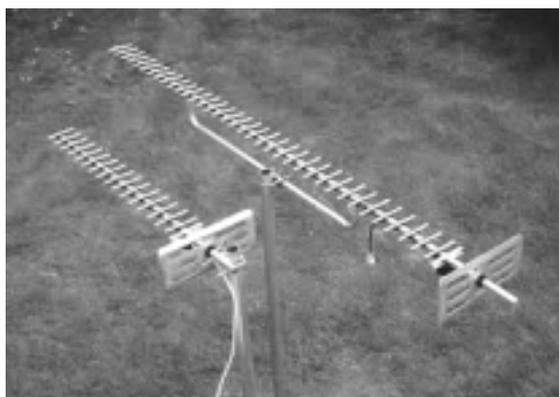
All of our 23cm aerials are specifically designed for ATV use – although they can be used for other modes as well. Wideband characteristics mean that you need only one aerial to cover the repeater input and output channels. Our famous wideband yagi's come fully-assembled in two versions:
