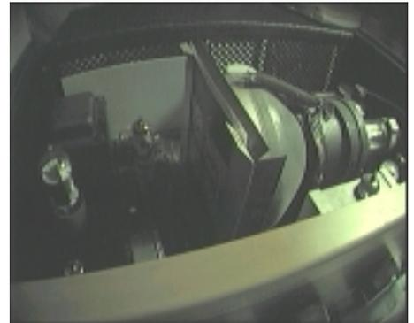
and cleaned all the PCB's with some switch cleaner. I then began to test it, feeding mains through a variac, to start with about 50 volts for an hour or so I gradually increased the supply, I saw the raster on the scanner - and a picture on the monitor connected on the video output.
