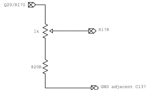
Connect other side of pot to ground via an 820R resistor.
