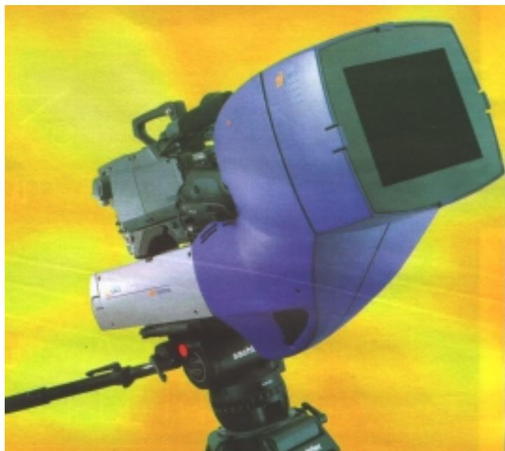
An Israeli company has developed a TV camera that can sense the depth of objects in real-time and so does away with the traditional blue screen background used for special effects.
