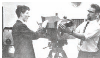
Andrew Tucker (l) and Terry Lane (r) adjusting Terry's image orthicon camera - Andrew's vidicon camera is in the left background
