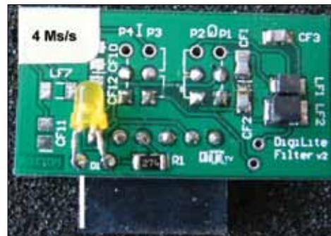
At the low cost of these boards it is tempting to use one pcb per Ms/s option and simply plug them in as required. In this case the links can be permanently wired. This option is not ideal however if the equipment is mounted inside a box.
