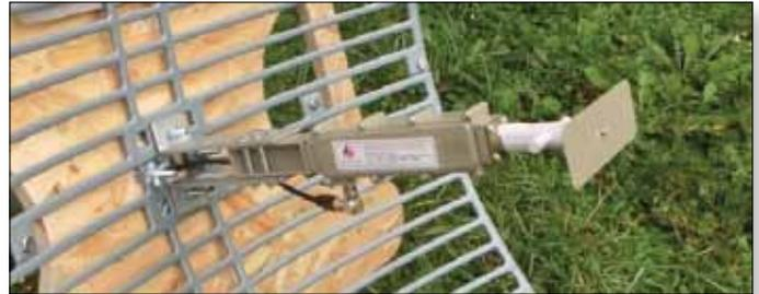
► Figure 3. MMDS LNB attached to grid-parabolic Wi-Fi reflector
