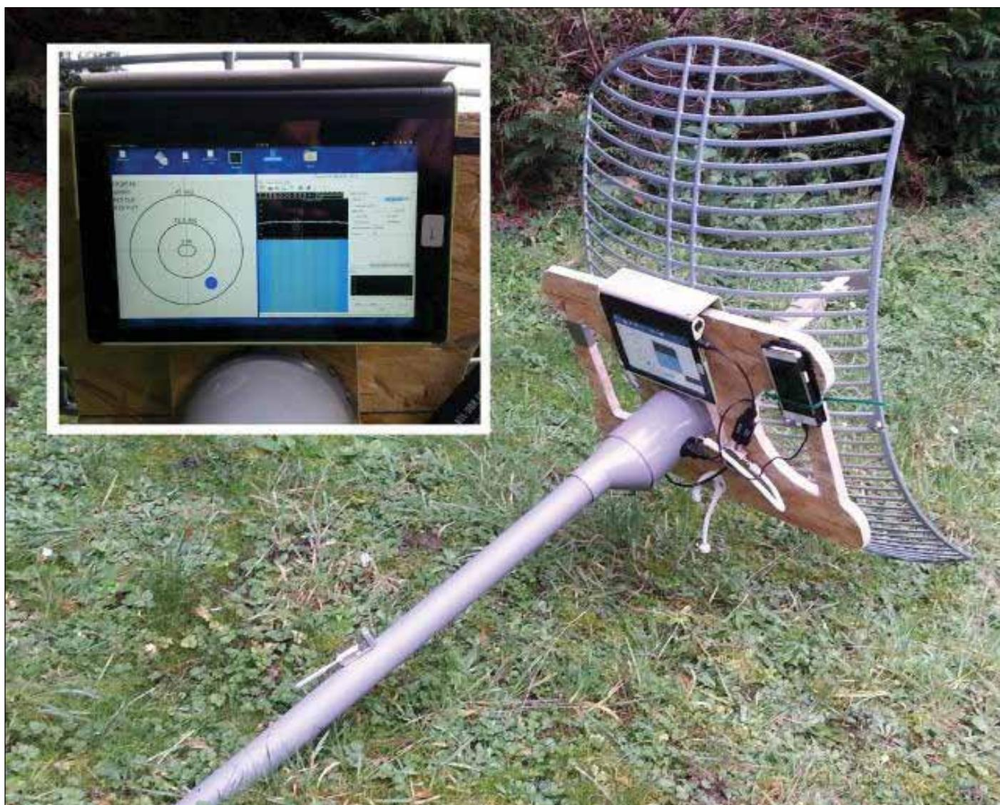
*A shoulder-mounted dish, tracking system and SDR receiver for amateur radio communications, originally designed for receiving HamTV digital video transmissions from the International Space Station.*
