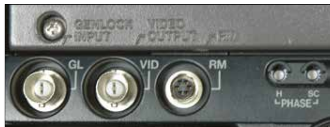
► Genlock & adjustments on a typical camera
