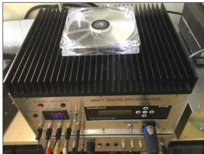
► Another view from the top showing heat sink and cooling fan for the power amplifier.
