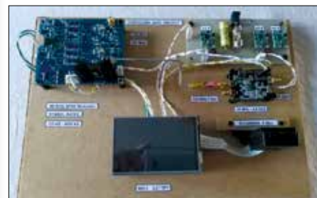
► Roland, F8CHK built this "open" Portsdown and labelled it for a demo at his local club. He soldered the filter-modulator board himself.
