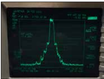
► Photo 3 Amplifier spectrum at Idq = 350mA Pout = +27dBm
