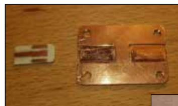
► Fig. 12 – EMM5074 pcb and its metal case.
