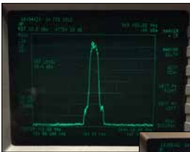
► Photo 1 DATV express drive signal +4dBm
