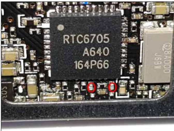
► Fig. 9 – Inside the VTX-HV. The two capacitors to be removed.
