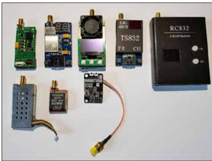
► Fig. 1 –Some of the FM-TV transmitters tested.
