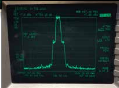
► Photo 2 Amplifier spectrum at Idq = 550mA Pout = +27dBm
