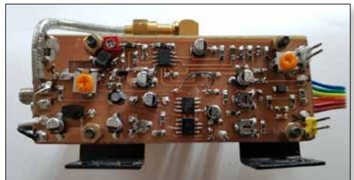
► Fig. 7- BANDABASE SMD pcb (layout by IW2FYT). Here it was used as a modulator of a 10GHz FM-TV exciter, firmly lodged in the rear.
