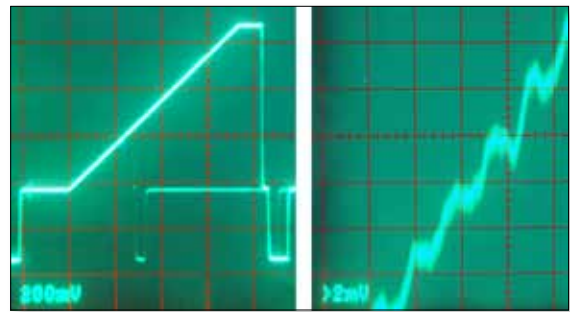
► Fig.2: This sawtooth is from a digital 8 bit test signal generator. However when you expand the gain by 100 times the quantization steps can be seen.
