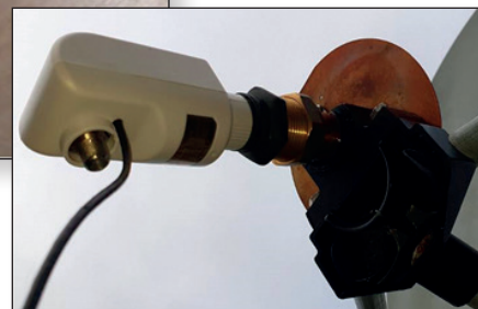
► Figure 5 – Compression fitting for a decapitated LNB
