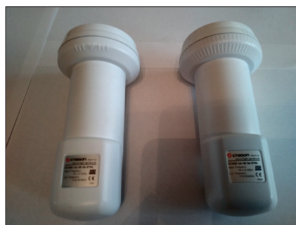
► Octagon twin output LNB OTLSO types, 27MHz left, 25MHz right. Notice the skew graduations. Photo G4HIZ
