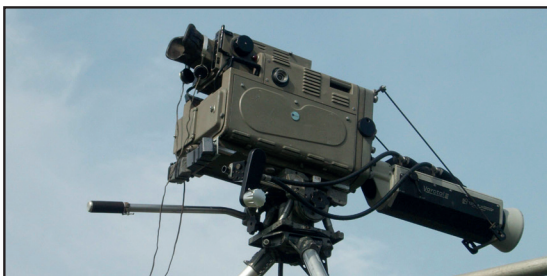
► Mk III fitted with zoom lens rather than the usual turret
