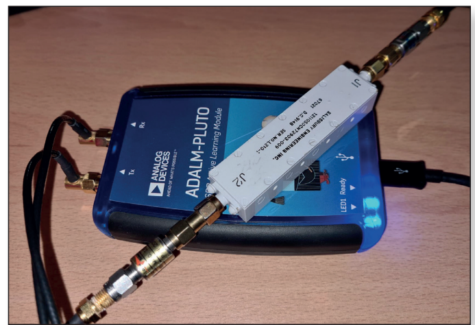
► Figure 2: PLUTO with X-Band Band Pass Filter connected.
