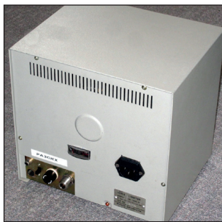
► Old monitor with a metal plate instead of the CRT
