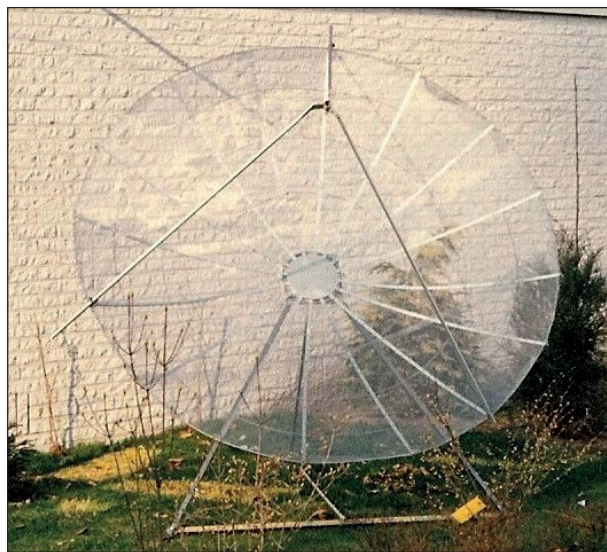
► Two-metre diameter dish for 11 GHz made by PA3CWS and PA3CRX
