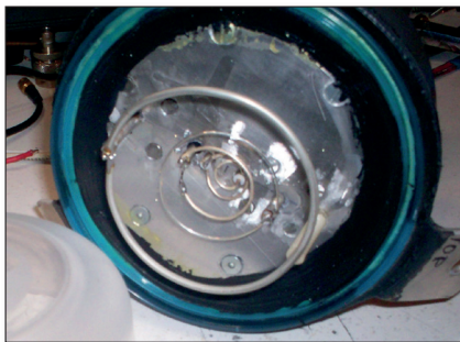
► Side view of the stacked ring feed developed by PE1CKK
