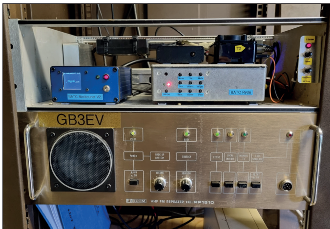
The AV output of the Ryde goes via a switching relay to a Pi3B+ running Portsdown 2020 software via an EasyCap.
