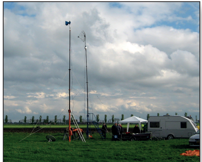
► The portable set-up in the field, the dish is under measurement. The reference horn was the subject in CQ-TV271.
