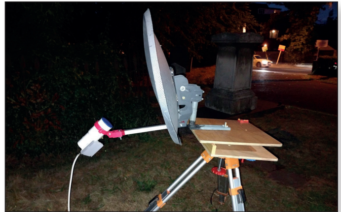
► Sky LNB showing a repurposed Sky dish and LNB mount, atop a 'Tilt-O-Matic'.
