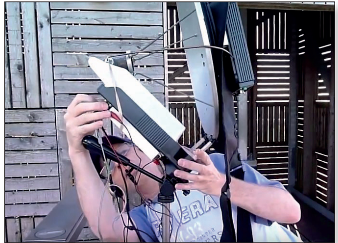
► 6 cm dish (with ATV station) on top of the 24 GHz ATV station
