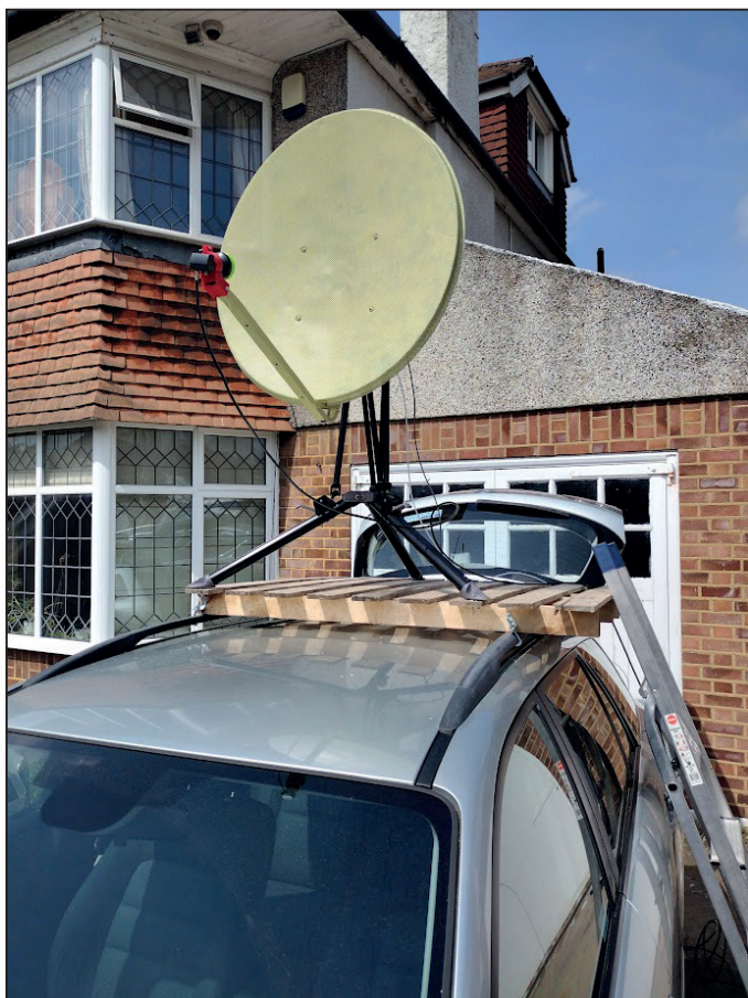
► Pallet, Tripod and dish all on the car roof. Side access via alloy ladder
