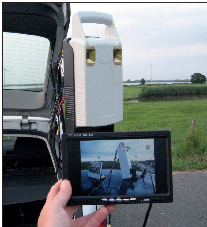
► Two horn antennas directly mounted on the Eyal-Gal module
