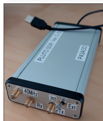
► Figure 6 The finished Hammond Box containing the modified Pluto
