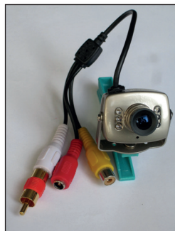
► My cheap IR camera, it contains even a microphone (the clamp is a clothespin)
